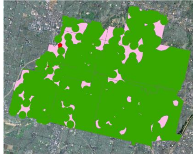
Macro + small cell coverage with optimally selected fiber access points as small cell locations
